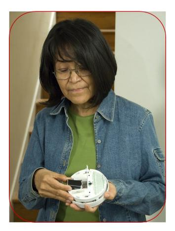
There are many brands of smoke alarms, but two basic types: <u>ionization</u> are quicker to warn about flaming fires and <u>photoelectric</u> are quicker to warn about smoldering fires.
